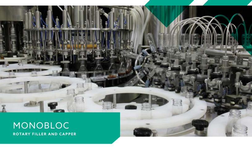
Volumetric, Flow Meter, or Level Filling Systems
